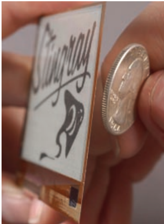
Figure 2: Gyricon's Paper-like Displays use Bichromal Microbeads
