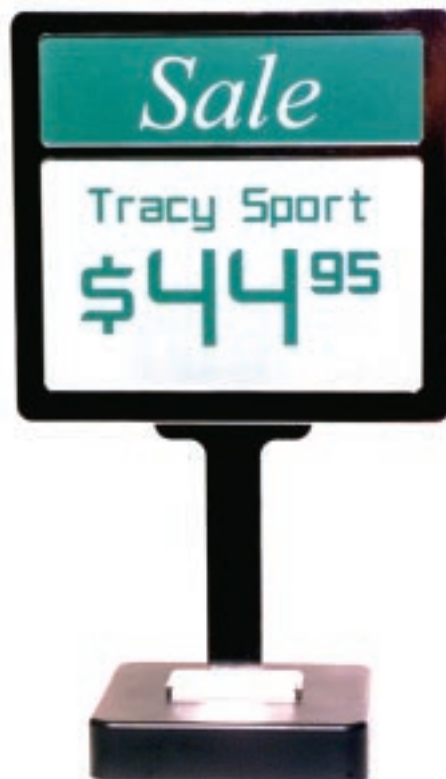
Figure 2: Gyricon's Paper-like Displays use Bichromal Microbeads
